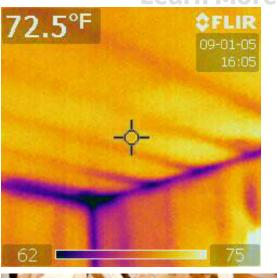
Infrared Camera indicates a lack of insulation in the attic.
